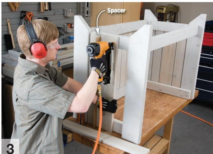
Attach the siding boards to the rails, spacing the boards roughly 1/4 in. apart. Adjust the position of the boards to keep them evenly spaced.
