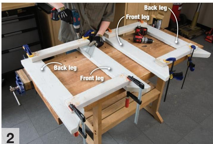
The side top rails are set back 7/8 in. from the front edge of the front legs. The side bottom rails are set back 3-1/4 in. from the front edge of the front legs. Both rails are 2-3/8 in. from the back edge of the back legs.
