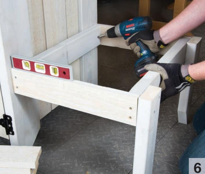
**Attach the side-shelf frame to the bench legs with 2-1/2-in. screws, keeping the top of the shelf level.**
