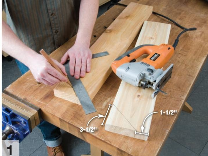
Mark the taper cut lines on the bench legs. Use a miter saw, jigsaw or handsaw to cut the tapers.
